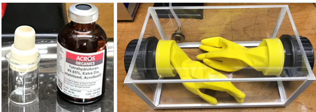
Figure 2: BDT molecules are handled and transferred to a glass vial in the glovebox under Ar atmosphere.
